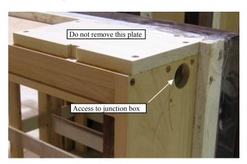
Step 2: A typical window as delivered from EG and equipped with an electrically heated I.G. unit. A wooden cover at the head of the window unit beneath the controller, must be removed to wire power into the unit. Remove screws shown and pull cover slightly down and toward you to remove.
